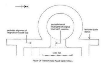
It seems therefore that when the nave was widened, a smaller original tower arch opening, approximately 3ft 4ins wide and central to the tower, may have been widened southwards to better relate to the wider nave. This was achieved by rebuilding the south jamb and leaving the north in situ; at the same time, the opening was heightened and given a pointed arch, and had there originally been an upper door to the nave, it would have disappeared within the taller arch.
